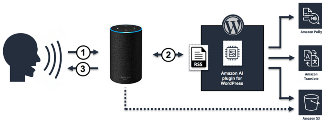
Figure 6: Flow of interactions required to expose WordPress websites through Alexa
